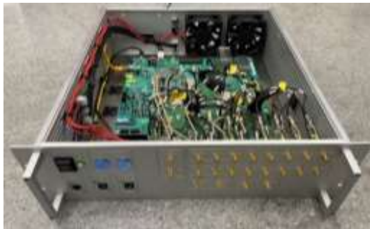
Fig. 2: The Xilinx RFSoc development board in a custom-made enclosure
